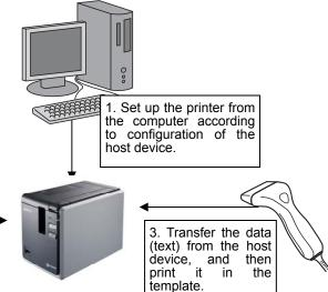
This allows the user to develop a printing system that connects directly from the host device. Compatible host devices are listed below.
